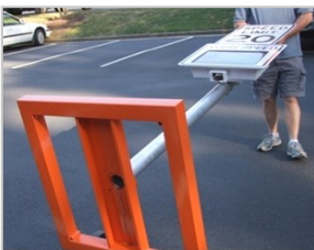
One-person operation to tilt and roll to a new location
